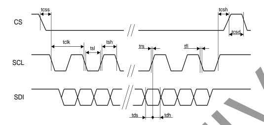
6.3.2 Digital RGB Interface Timing Characteristics
